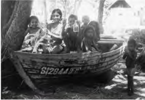
A bakkura . The small but sturdy local dinghy. Maldivian vessels were built without plans but with utmost care. While the boat was being built, the master carpenter would turn around it holding a length of rope or a palm leaf, taking measurements and giving instructions to the carpenters.
